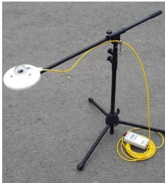
Fig.4.1 Single-headed pyranometer (a, c), Data Logger (b, d) (The value on the screen is based on W.m^{-2} ).
